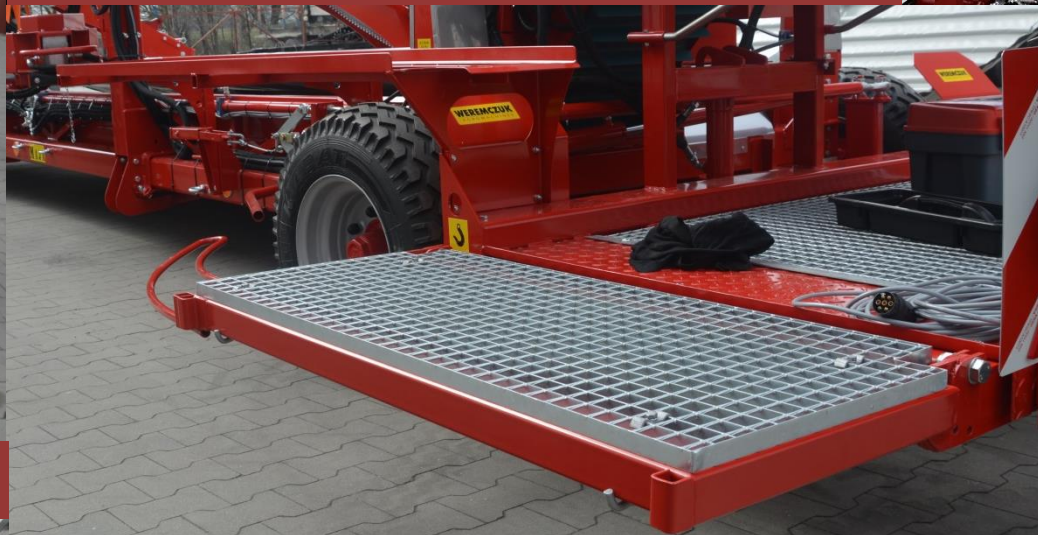
Additional side work platform
