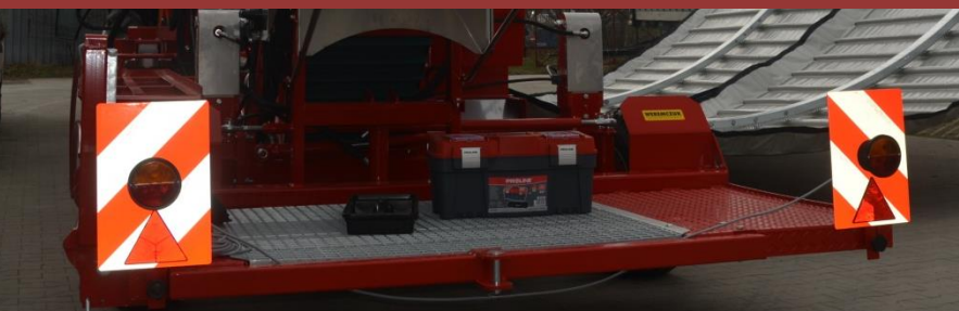
Road lights with white-red boards
